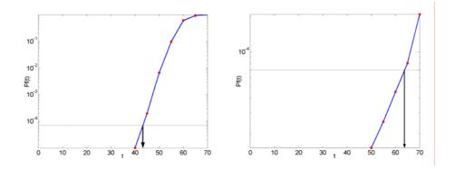
Fig. 3 The curves of probability of failure: (a) member without secondary protection, (b) member with the two secondary protective paintings
